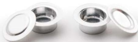
The qualities of a “good” DSC measurement with respect to sensitivity, resolution, baseline stability, etc., are usually attributed to DSC instrument performance and rarely to sample preparation and choice of crucible. Nevertheless, the latter two details also play a decisive role in the quality of the measurement. The choice of crucible, in particular, is key to achieving reproducible DSC measurement results.
