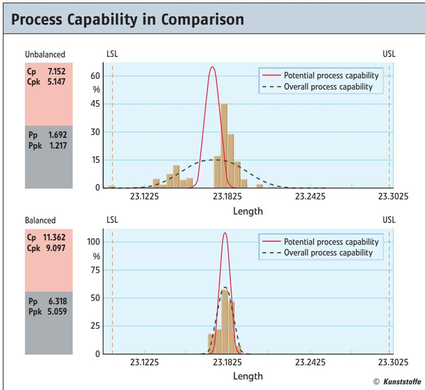
**Fig. 4. Potential process capability and overall process capability, expressed in terms of the length of the sintered ceramic bodies. This overall process capability improves from the unbalanced to the balanced state by more than a factor of 4 (figure: Philips)**
