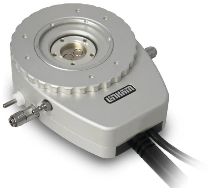
Figure 1 – DSC450 stage with sample and reference position.
